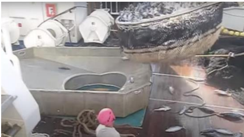
Figure 6. Large hopper tray lacking a stop door to avoid bycatch moving too quickly into the lower deck.
