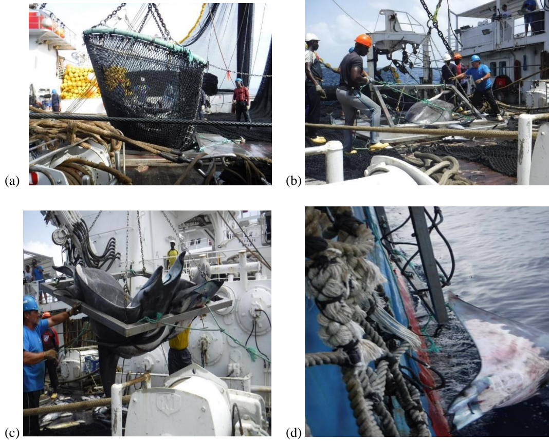
Figure 4. AZTI manta sorting grid use release steps: (a) empty metal grid contents into unloading hatch, (b) connect grid frame with chains to deck crane, (c) move sorting grid towards starboard railing, and (d) release animals into the water.
