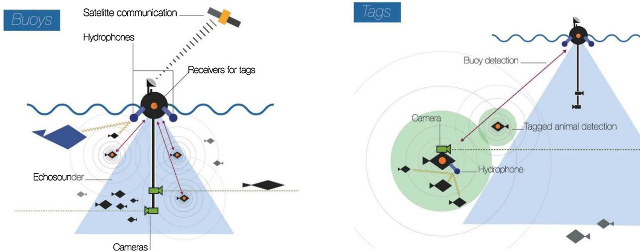
**Fig. 3.** Schematic diagram of the nodes that would form the observational network: buoys and tagged fauna.
